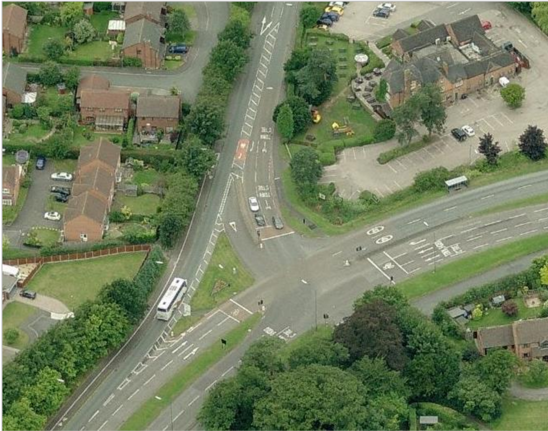
Figure 2-11: Shelton traffic signals – the cycle lanes do not continue along A458 Welshpool Road (Source: Bing Maps)
